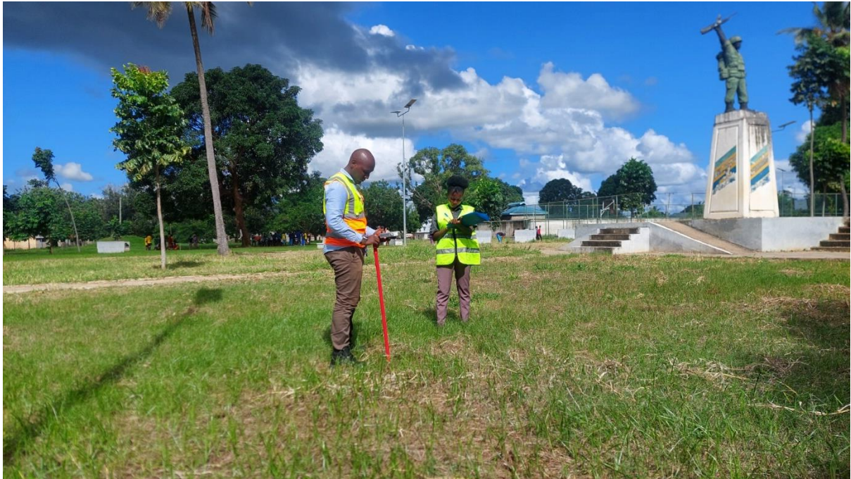
Picture 2: Ambient Radiation Measurement at the environment of Mashujaa Park – Mtwara
